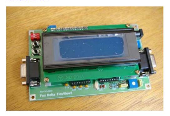
FOXVIEW3 Rev0511 is last revision of FoxView series of APRS Viewers for radio amateurs, based on original design by Max/IK3SVW's Peek\_SVW.
