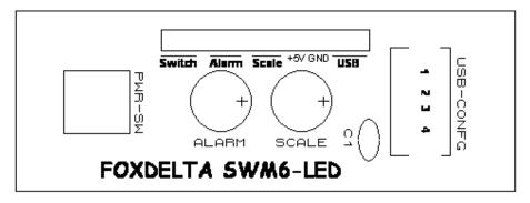
This board has a power ON/OFF switch, USB connector and two Dual LEDs for Scaling indication and "Alarm"
