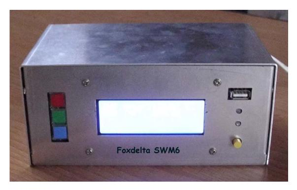
SWM6 is an USB / DC12V Powered SWR Meter, a project Based on Microchip's PIC18F4550.
