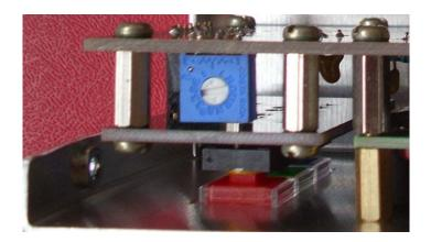
A Contrast preset (P1) is provided and must be adjusted until you see characters on LCD.
