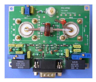
Dual Scale HF Bridge has two scaling relays under CPU control.
