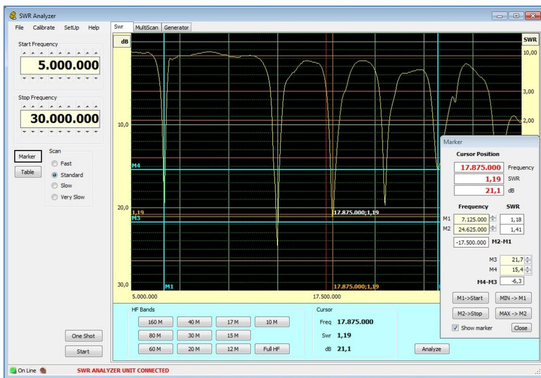
If the Start or Stop frequency has been changed during the continue analysis phase, the graphic can be updated to the new frequency range, pushing the “Refresh” button that will appear changing the frequency .
