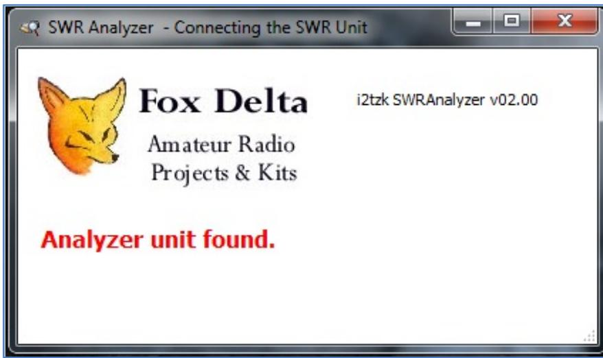
When program starts, it automatically searches for the SWR Analyzer board exploring all the USB devices.
