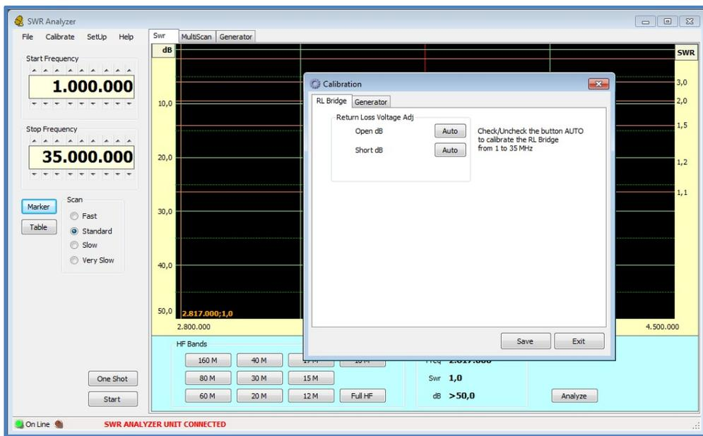
Be sure that *no cable is plugged* into the Antenna connector, select the option “Open” then run the automatic calibration process by pushing the button “Start”.
