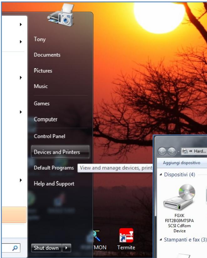
Driver installed can be verified selecting “Device and Printers” from the “Start” menu (Windows 7) or from the “Control Panel”
