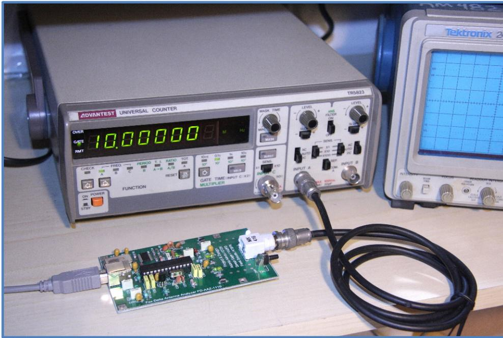
Connect the antenna output to the frequency meter.
