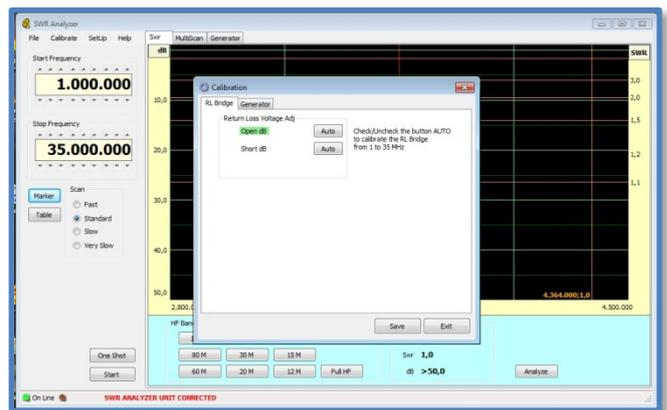
Select now the “Short circuit” calibration and connect a *0 Ohm terminator* to the Antenna input.
