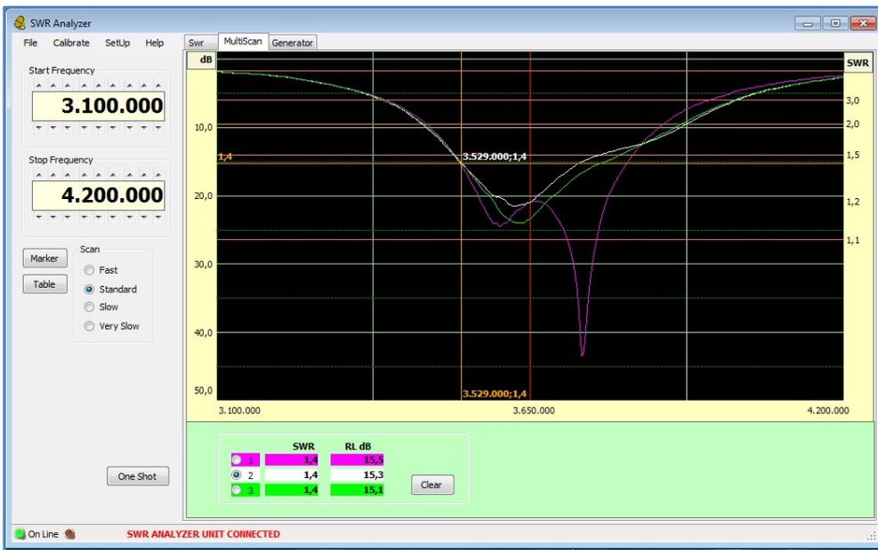
Pass band filter response to open, 50 ohm and 25 ohm terminator.
