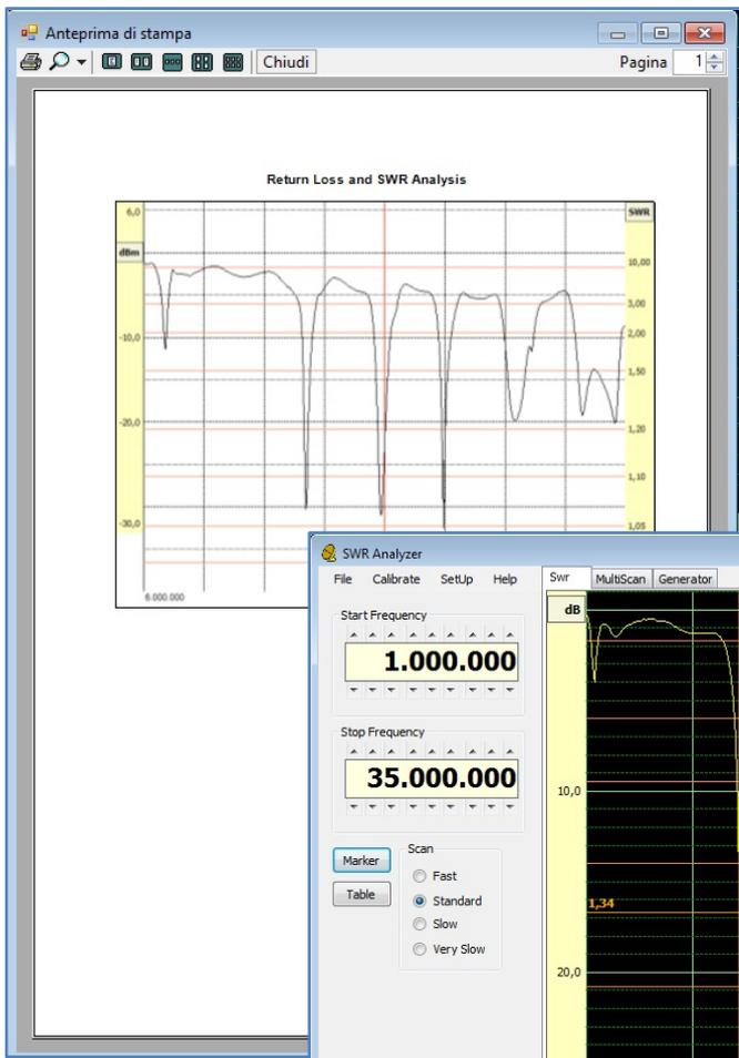
The PC program, Windows based, allows to explore a single HF Band or the full range from 1 to 35MHz and plot the resonance figure.
