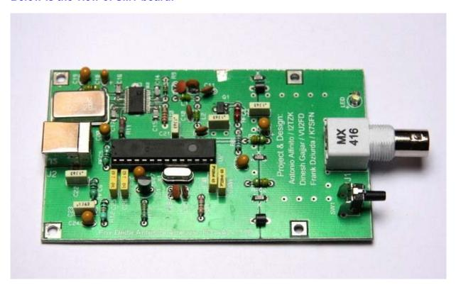
Final version of Antenna analyzer uses AD9851 carrier board where AD9851 may be supplied presoldered and a DIP8 package for AD8307:
