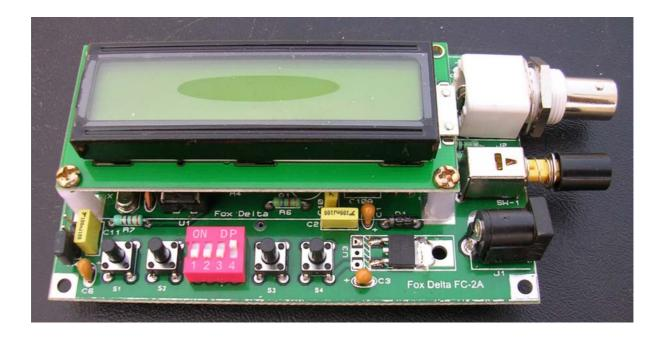
This Frequency counter Project is based on PIC16F84A Micro controller chip manufactured by Microchip. Although rated at 1.1GHZ due to Pre-Scale IC capability, it can measure up to 400MHZ in this project.
