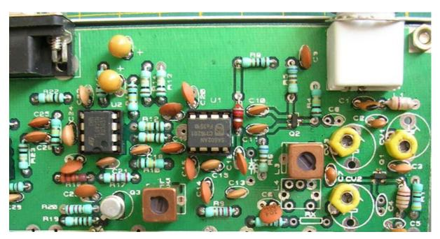
Galileo uses dual J310/309 FETs as front end. The First FET is used in Grounded Gate config and matches the Dipole antenna at source.
