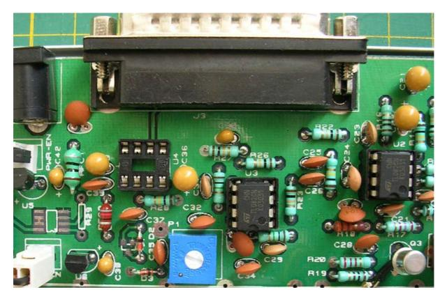
Galileo is ready for data transmission. It uses a Maxim MAX187 A to D converter chip. Data output is available at the back of the receiver thru a D25 Parallel Port connector.
