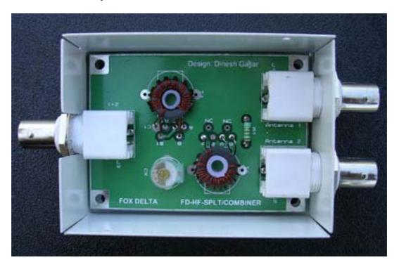
2. Two Antenna Balun for center feed Dipoles
