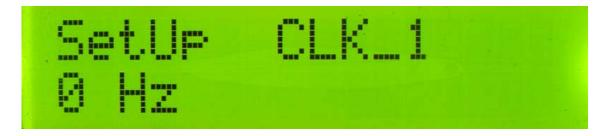
Si5351 module has second signal available at CLK1. May be used for Second IF in a receiver or Transmitter.
