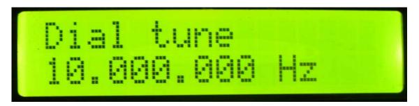
Use the rotary encoder to change frequency
