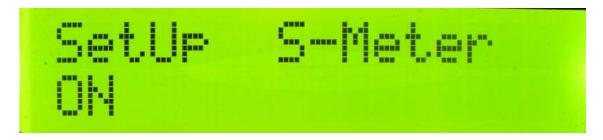
Select ON or OFF. This activate PIC PIN2 for analog DC signal for measurement of S-Meter or ALC signal level and display it in Bar Graph form on LCD. (DC 0 to 5V)
