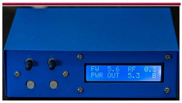
Front Panel Switches: Power ON/OFF (Left) Battery/USB Power (Right)
