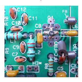
Q1, RF Amplifier is SMT part and is Pre-Soldered on board for Kits.
