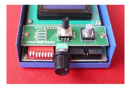
DIP SWITCH: switch configuration is read once at start up, so changing any switch takes effect resetting the unit.
