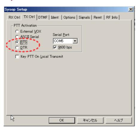
TinyEcho may be powered by DTR line if it is made "Active". With script running, DTR line will remain high & provide required power to the interface.
